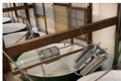
Mixing moromi in a fermentation tank with a bar
